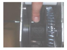
30. Maintain the CBLM block plate when turning the drum down until the strap is completely wound up around the drum, then release the CBLM block plate.
