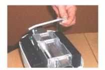
10. Remove the batteries and pull contact plugs.
