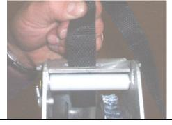
25. Pass the strap under the strap roll, and pull it as shown below.
