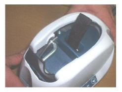
14. Slightly lift the main cab to free the touch pad membrane then unplug it from the main circuit board.
