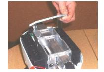
9. Remove the batteries and pull contact plugs.
