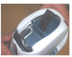
13. Slightly lift the main cab to free the touch pad membrane then unplug it from the main circuit board.
