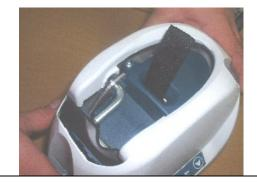
13. Slightly lift the main cab to free the touch pad membrane then unplug it from the main circuit board.
