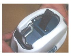
13. Slightly lift the main cab to free the touch pad membrane then unplug it from the main circuit board.
