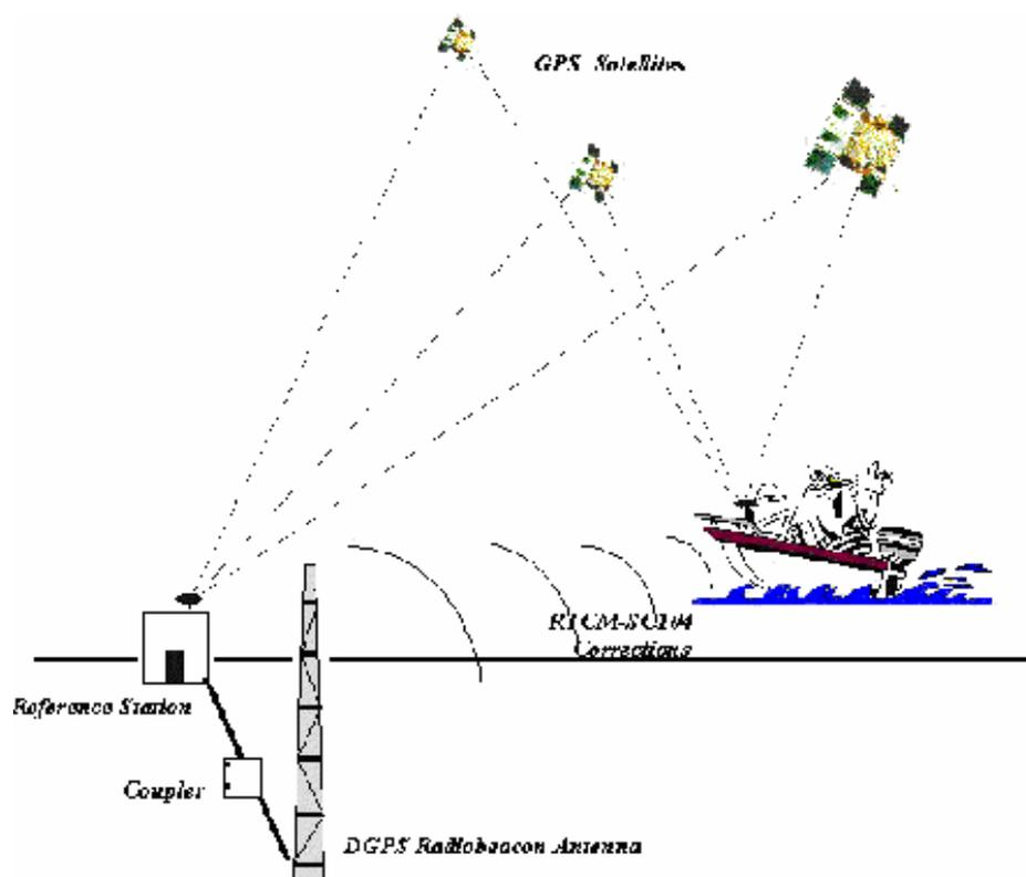
figure 25: Basic sketch of the DGPS system
