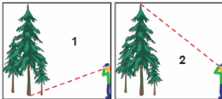
**figure 104: Pointing towards birch point & top of the tree**
