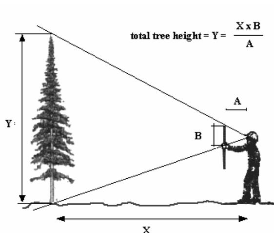
figure 42: Height measurement based on geometric principles (similar triangles)
