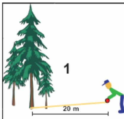
**figure 102: Measuring the distance to the tree**
