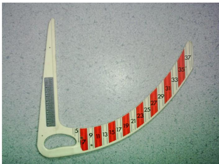
figure 41: Example of a tree calliper
