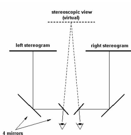
figure 40: Schematic view of a stereoscope
