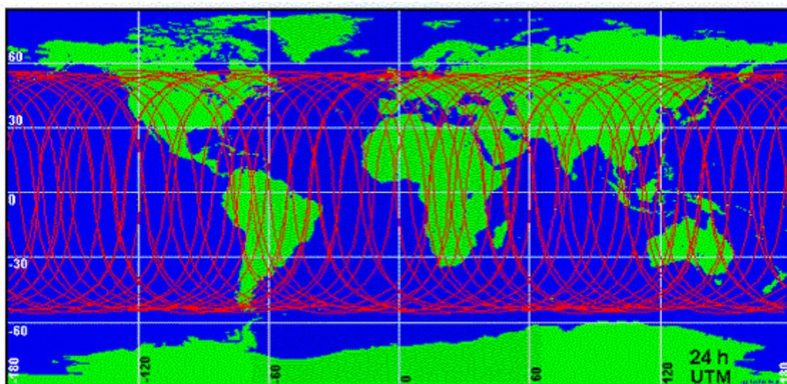
figure 23: Satellite routes projected on the earth surface
