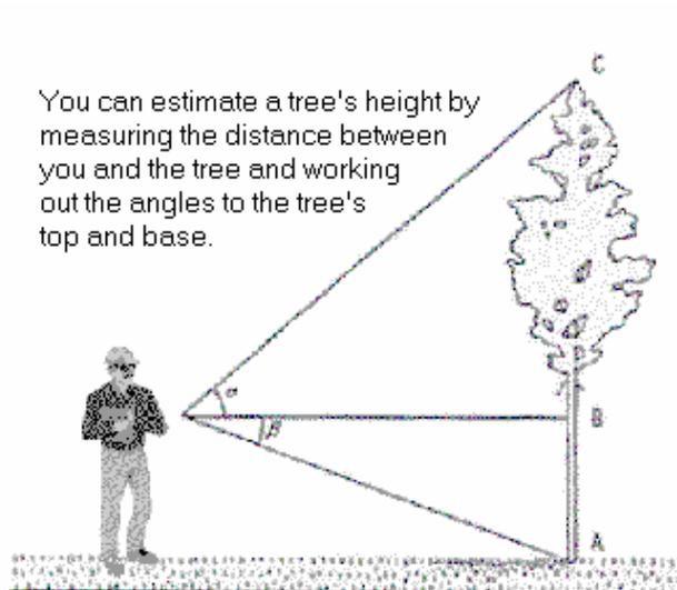
**figure 43: Height measurement based on trigonometric principles (angles)**
