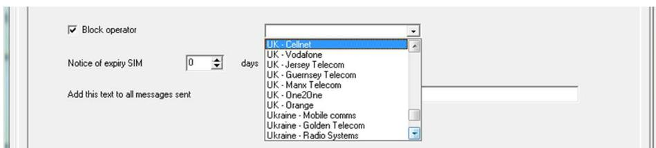
4. **SIM Expiring Warning** > countdown in days after which the panel will send an alert of “SIM expiring”. This option help the user to renew the SIM contract or charge credit maintaining the SIM active.
