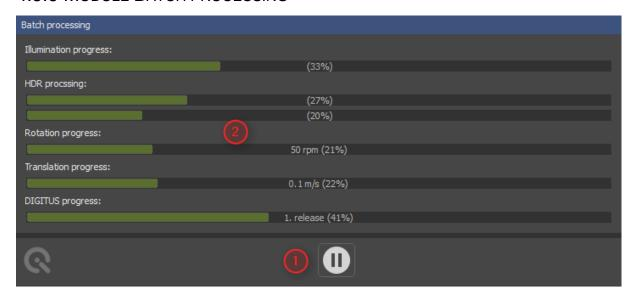
If at least one batch table is activated, the process is started by clicking the *play/stop* button [1]. Clicking the *play/stop* button again immediately stops all processing after confirmation.
