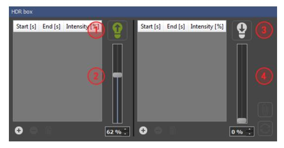
The HDR option module in the software enables you to control both LG2 lamps of the HDR box. The upper lamp is switched on with the *up* button [1] and the intensity controlled with a slider or an input field [2]. The same applies to the lower lamp [3, 4].
