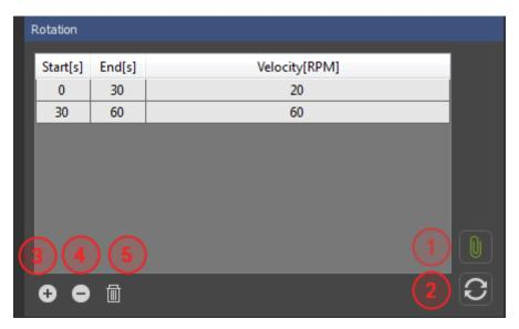
Each module in the software, except the timecode display, has five buttons and a table for batch processing. Tables for sequences of movements, rotations, DIGITUS releases, and illumination (lightHEAD and HDR option) can be edited, modified and saved for reuse. All batch tables can be executed simultaneously.
