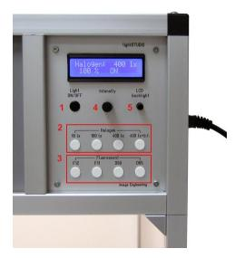
For the initial operation, select a light source by using one of the push-buttons [2, 3] after turning the power supply on. Press the button "Light ON/OFF" [1] to illuminate the corresponding light source.
