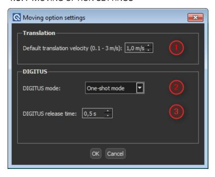
In the *Moving option settings* dialog, specifications can be modified for some components of the MOVING lightSTUDIO.
