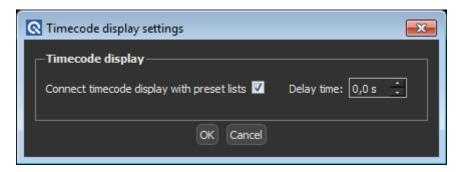
The *Connect timecode display with batch lists* option allows the time code display to start simultanously with processing start. The delay time defines a time lag after which the display starts. The starting time is the value entered in the fields in the corresponding module (see chapter 4.5.4).
