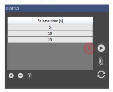
The DIGITUS device allows you to release your camera button with the software. You can release DIGITUS with the *play/stop* button [1] depending on the settings in the options menu (chapter 4.3.1) in one-shot, toggle or continuous mode. A status bar at the bottom displays the continuation of the DIGITUS in released state. During batch processing, the *play/stop* button is disabled. In the batch table time stamps for the release of DIGITUS can be edited. At each time stamp DIGITUS is released
