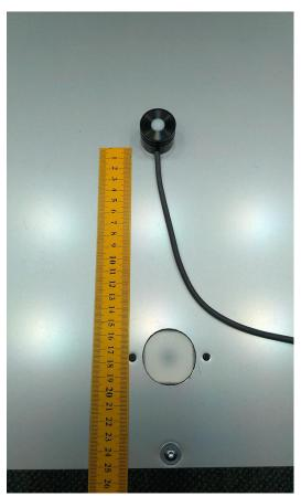
of the bottom plate (approx. 25 cm from front side, see image on the left). These two factors, the geometrical deviation and the loss of light caused by the glass, can be corrected by measuring the illuminance with a luxmeter.
