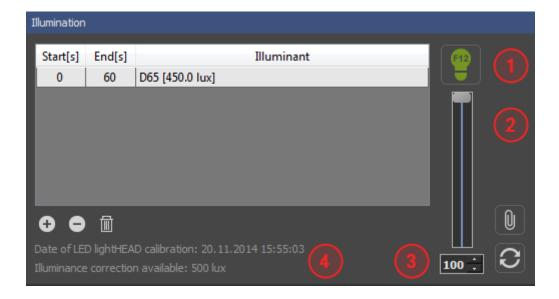
Besides the iQ-LED technology there is also a F12 lamp mounted into the LED lightHEAD. Thus this lamp can be switched on and off with button *F12* [1] and varied in intensity with a slider [2] and an input field [3]. During processing a batch this lamp is turned off in order to attain the selected spectrum and illuminance (in the example above D65 and 450 lux).
