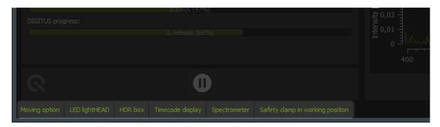
The status bar gives information about the connected hardware devices. If a component is available in your lightSTUDIO configuration it is highlighted in green. The release state of the safety clamp is also displayed.
