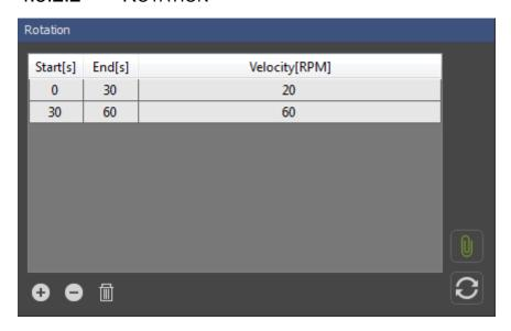
In the batch table, sequences for the rotating chart can be edited. There are three columns available, the first sets a start-time, the second the end-time for a period of rotation and the last column the
