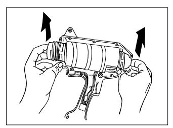
**9.** Grasp the faulty heat tube by the metal ends and lift it out of the lower housing. Avoid handling the insulation wrap – see below.
