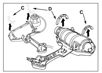
7. Remove the upper front standoff (C) and rear standoff (D) and set aside for reassembly. The standoffs might be found either on the heat tube or in the upper housing.
