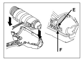
**10.** Hold the replacement heattube by the metal ends, aligning the keys (E) with the recesses (F) in the standoffs and push down into place. If necessary, rotate the heat tube slightly, to make sure the heattube is fully seated into the standoffs.
