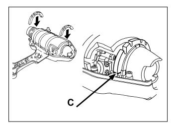
**13.** Place upper standoffs into grooves in heattube, making sure keys in heat tube are fully engaged in recesses in standoffs. Upper and lower sets of standoffs should be in contact with no visible gaps between them at all four locations (C).
