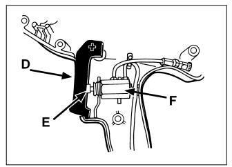
**14.** On the upper housing, make sure the trigger (D) is engaged on the valve button (E) and the trigger is positioned properly in its bearing.
