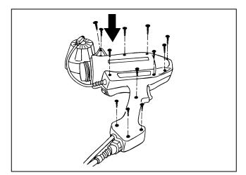
**18.** Recheck proper fit and alignment between the housing halves and make sure the trigger pivots freely.
