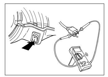
**12.** Check for proper electrical installation by connecting a multimeter or continually tester across the power cord plug blades. Continuity should exist when the switch is pushed to the on position.
