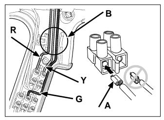
**11.** Route the wire leads as shown. Hold wires gently with a needle-nosed pliers to obtain bends.
