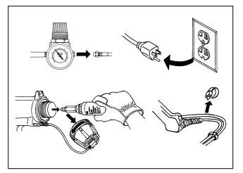
**1.** Disconnect air and electrical power and allow the applicator to cool to room temperature before disassembly.
