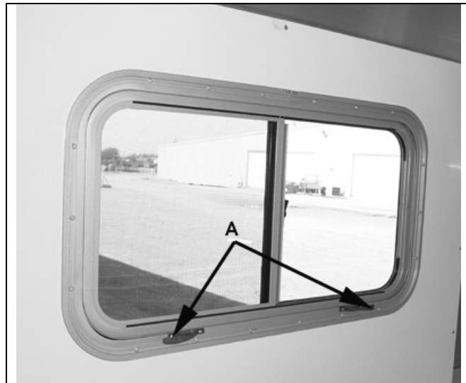
Figure 8-6 – Egress Window Latches
