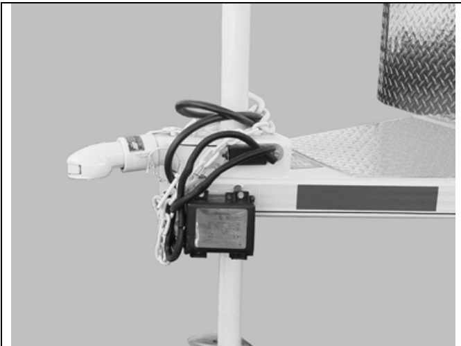
Figure 4-3 –Tagalong Trailer With Ball Coupler
