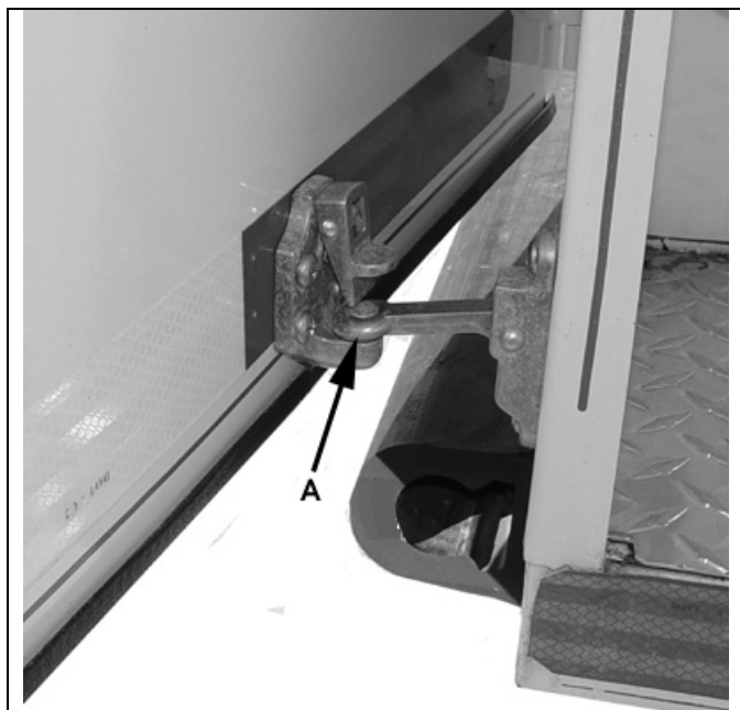
Figure 5-1 – Right Side Door Holdback
