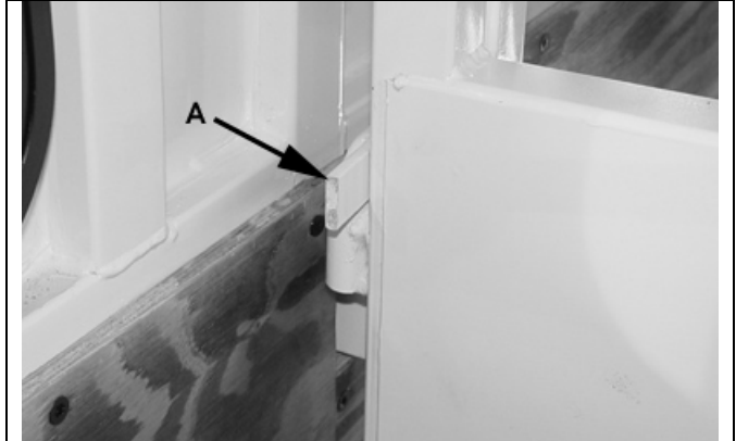
Figure 8-2 – Center Gate Latch
