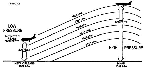
Figure 10-1.-Altmeter errors due to change in surface pressure.
