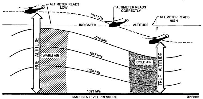
Figure 10-2.-Altimeter errors due to nonstandard air temperatures.
