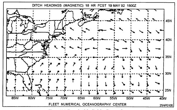
Figure 10-3.-Example of the ditch headings product.
