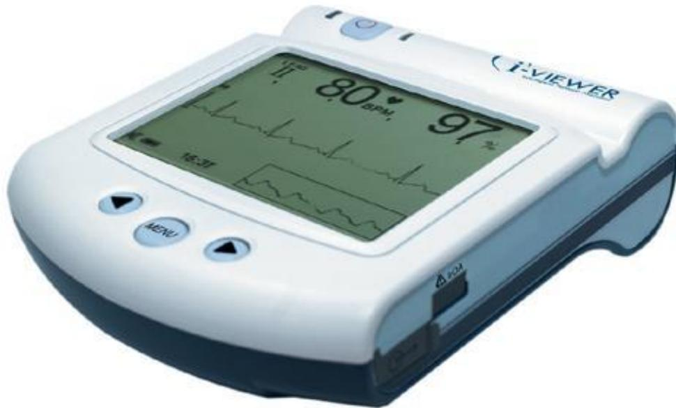
The i-Viewer CU-PH2 is a lightweight, portable, battery operated, 5-lead Electrocardiogram (ECG) and SPO2 monitoring device.
