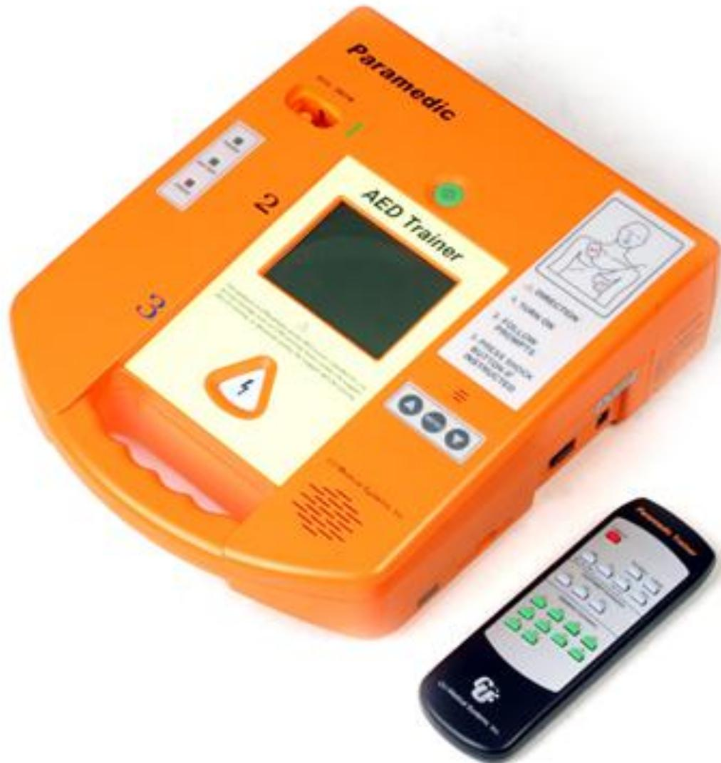
The CU-ERT is a defibrillator simulator designed to mimic the operations of the Paramedic CU-ER1. It can simulate all the functions of the Paramedic CU-ER1 including charging and shock delivery.
