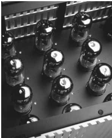
Beneath the S-400's top cover. The green LED lights beside each tube confirm status and blink to indicate a bias adjustment is underway.
