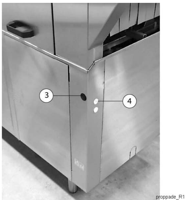
Plugged holes for hoses for detergent and drying agent
