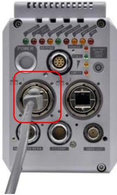
Insert the LAN cable into the "GIGABIT ETHER 1" connector.
