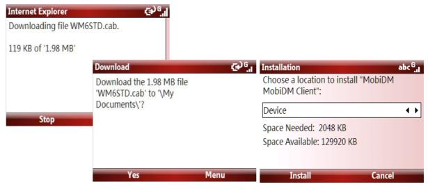
If this screen is shown, click on Yes to confirm installation. A cab file is downloaded and the applications will be installed on your device.
