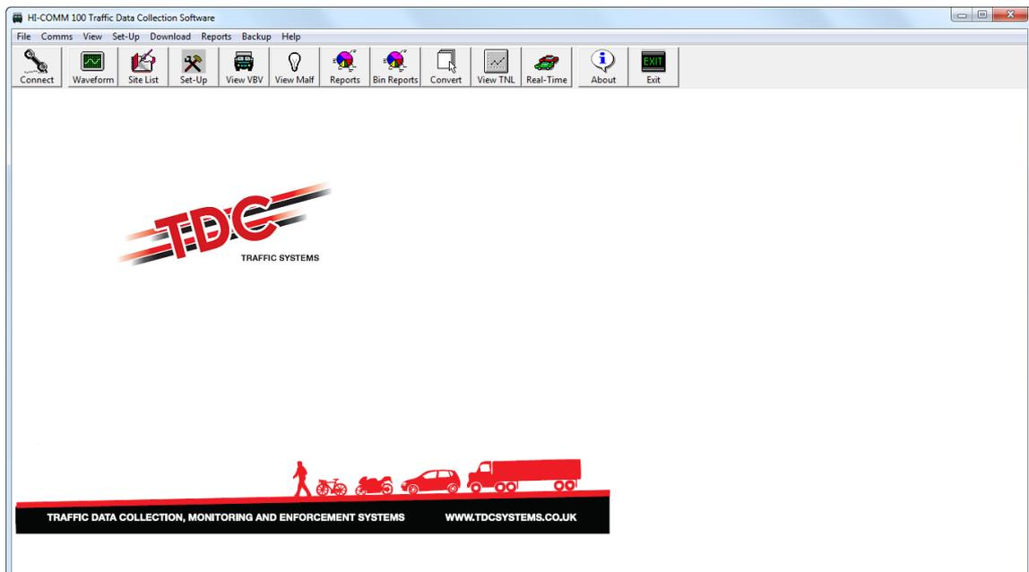
6. To set up a new HI-TRAC site select **Site List** from the tool bar; this opens the **Append HI-TRAC Site List** from which you can create a new site for your HI-TRAC installation.
