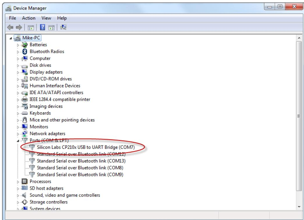
If you need to change the designated COM Port the right click on **Silicon Labs CP210x USB to UART Bridge (COMx)** and open **Properties**. Note the example below states COM7 but your PC may indicate a different port.
