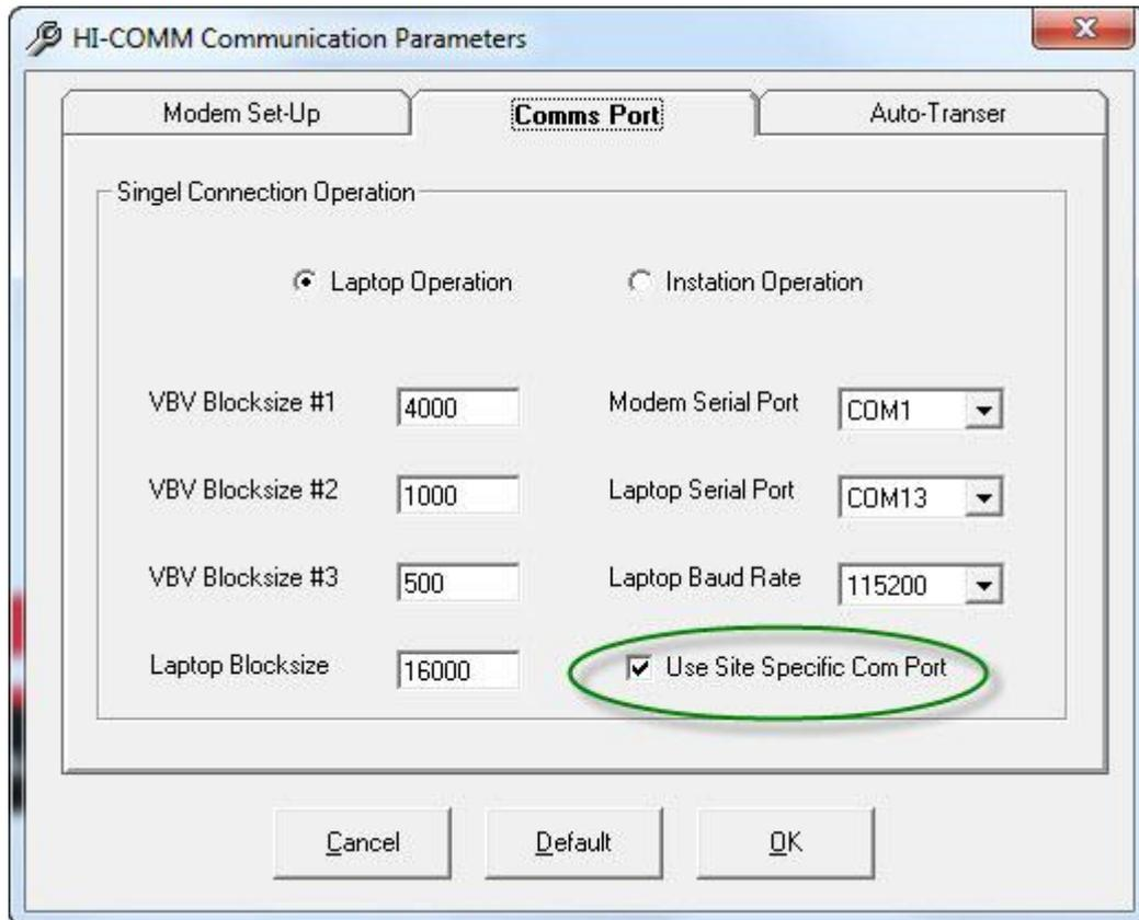
6. If selecting Site Specific Com Port ensure that the communications port setting in the site details is the same as the port shown in Device manager when connected via a USB cable.
