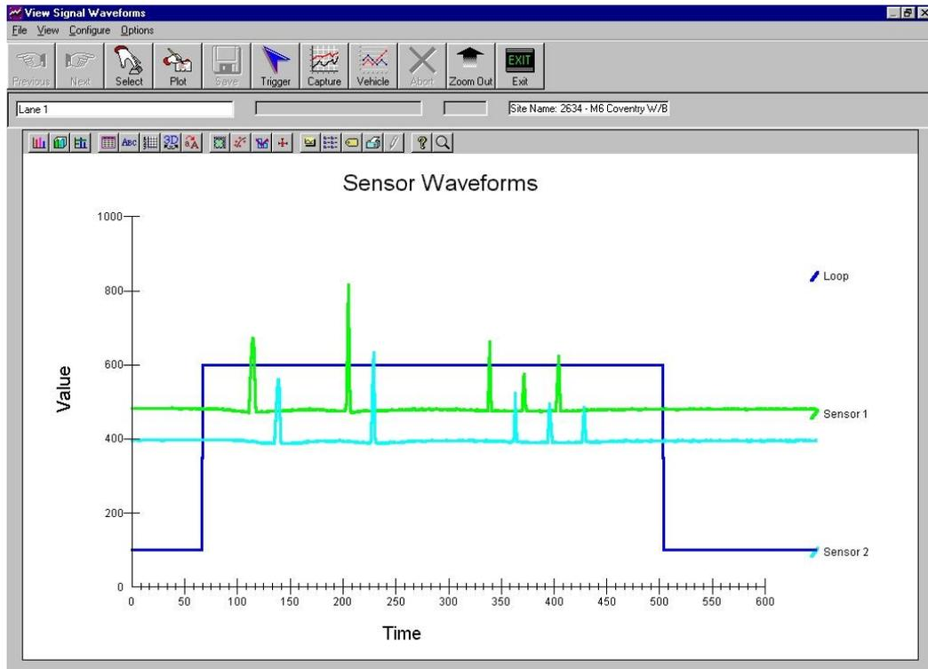
When connecting the HI-TRAC® EMU3 to sensors for the first time, perform a sensor test for approximately 100 vehicles and view the results. If the sensor counts are to within +/- 10 % and the loop and vehicle counts tally, the sensors signals are probably good. (Beware of straddling vehicles, they have the effect of increasing the loop count above the vehicle count as they are only recorded as a vehicle in one lane but activate the loops in two lanes.)
