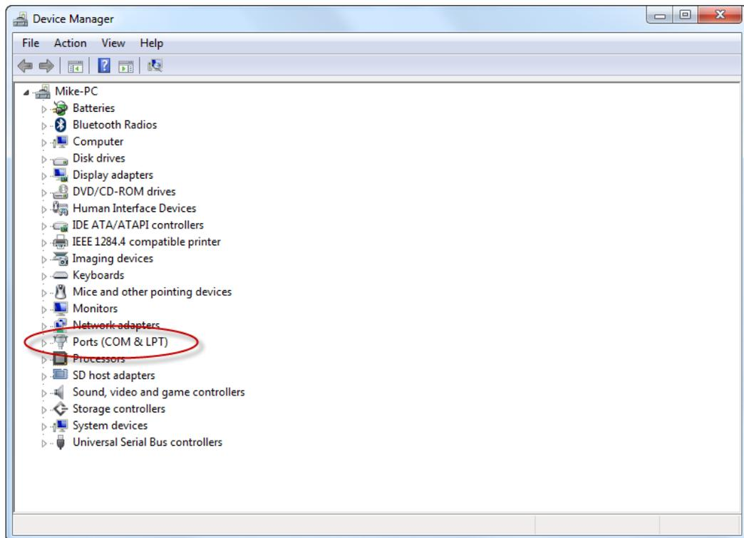
Note the COM Port designated to the USB UART Bridge; in the example below it states COM7. This is the COM Port your HI-TRAC will use to connect to your PC running HI-COMM 100 software. Make a note of the designated COM Port.
