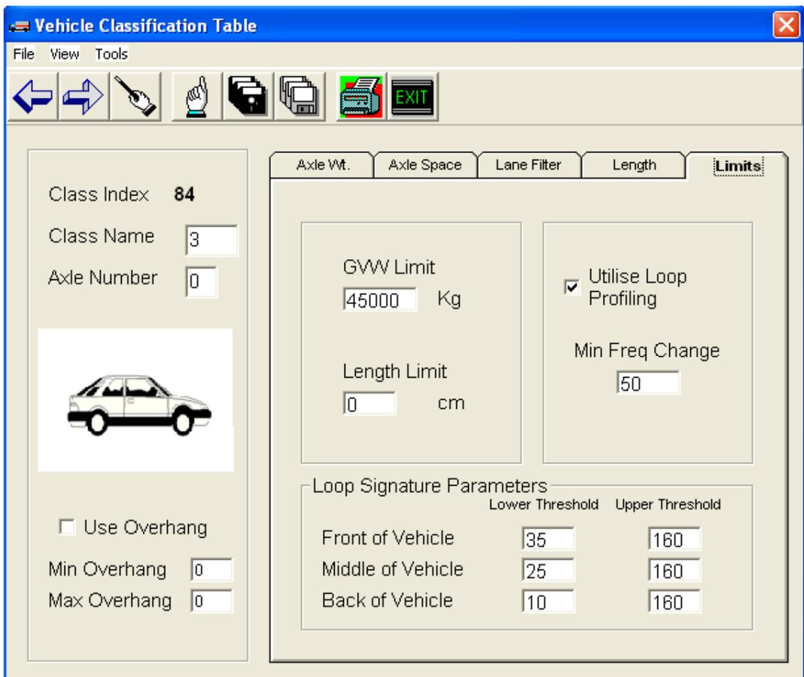
For a vehicle to be classified as a class 3 the frequency profile must comply with the following:
