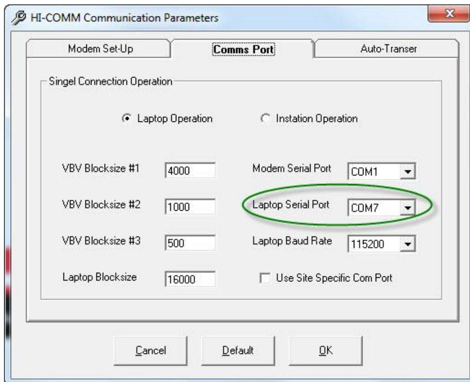
3. Select the Laptop Operation option and set the Laptop Serial Port to the serial port indicated in Device Manager and set in the Append Site List site set-up details (e.g., COM 7).
