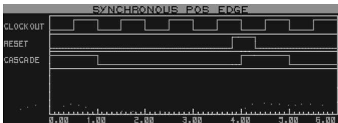
*We are clocking internally at 1Hz. Note that the clock is unaffected by the trigger and that the trigger actions on the falling clock edge subsequent to the positive edge pulse.*
