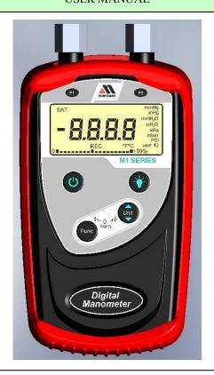
Meriam Process Technologies' M1 Series pressure instrument is a microcontroller-based pressure sensing device that can be used to directly measure pressure. Differential, Gauge and Absolute pressure sensors are supported up to 100 PSI. Pressure can be displayed in selectable engineering units of PSI, bar, mbar, kPa, mmHg, inHg, mmH2O or inH2O.
