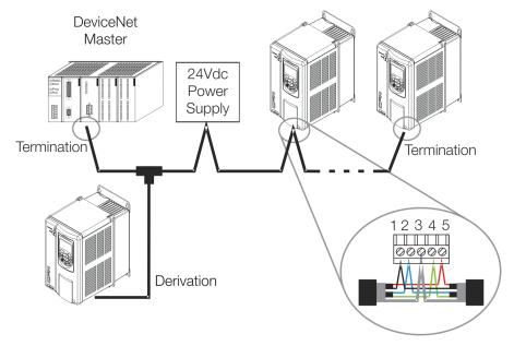
Figure 3.2: DeviceNet network installation example
