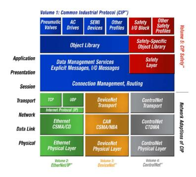
Figure 1.2: CIP protocol structure in layers
