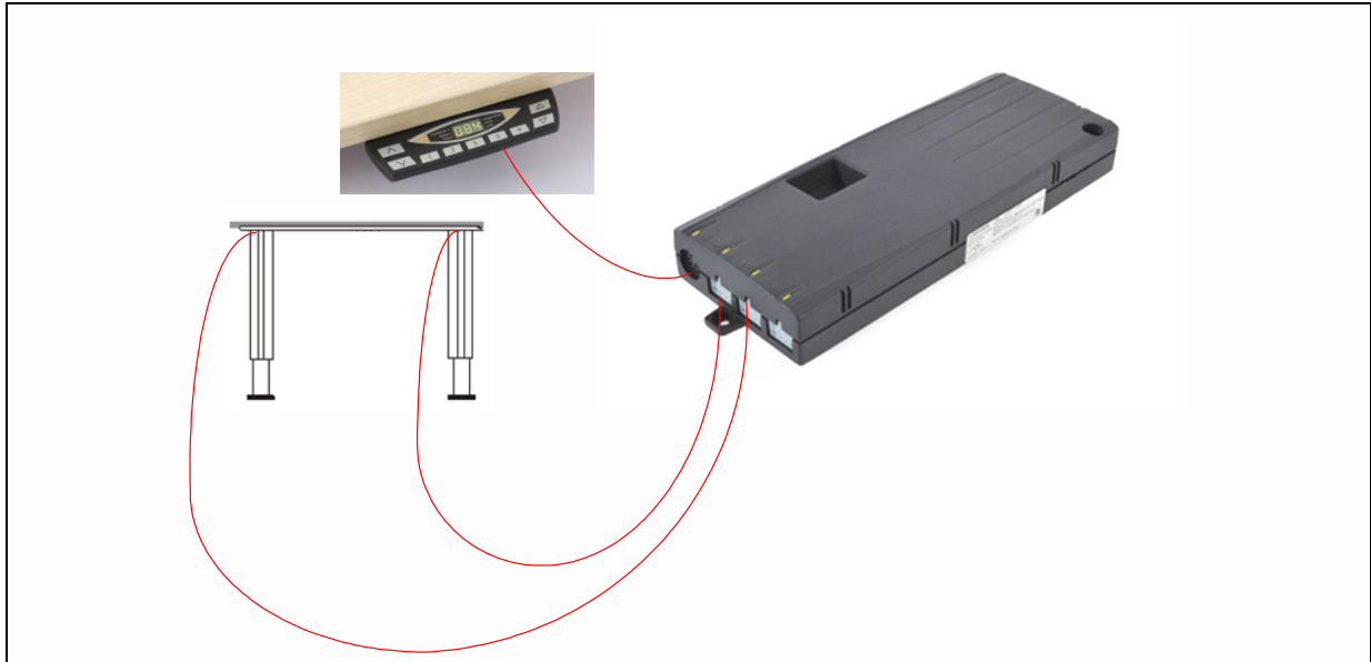
Figure 4: Connect the HSF cable-handswitch to the control box (e.g. COMPACT)
