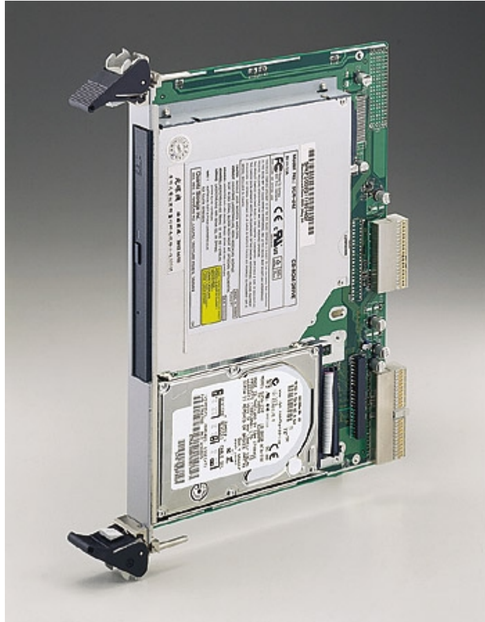
Figure 2-4: Installing 2.5" hard disk drives and slim CDROM
