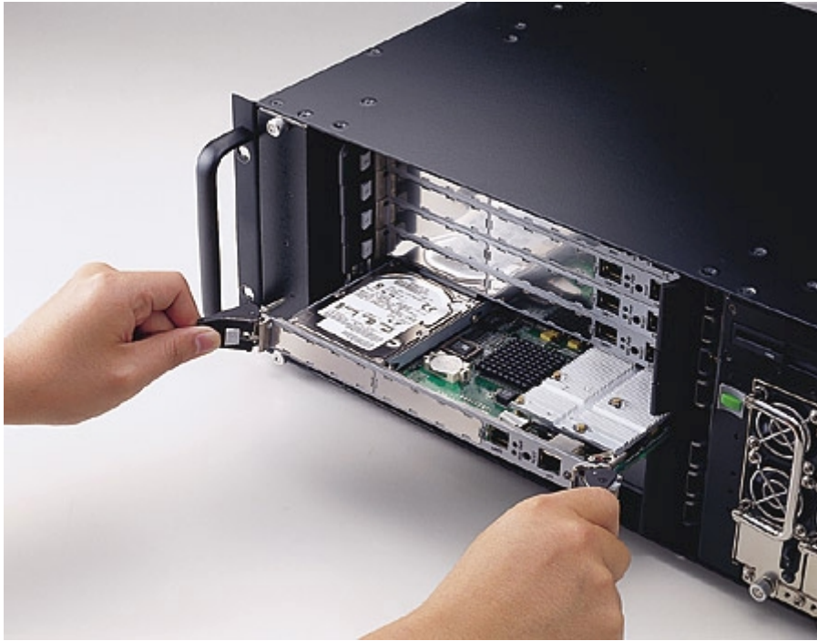
Figure 2-3: Installing a card into the chassis
