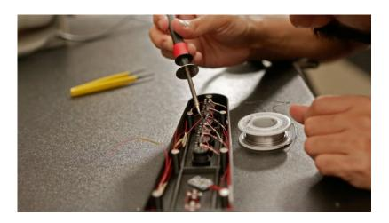
There are 70+ solder points in the complete circuit. We're using 30 gauge wire, which is ideal for working with small solder points.
