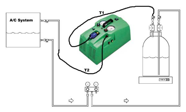
Before use, make sure that all the flexible hoses, the filter drier, the stockage-cylinder and the recovery unit have been in advance evacuated or that they contain the same refrigerant as the one to be transferred.
