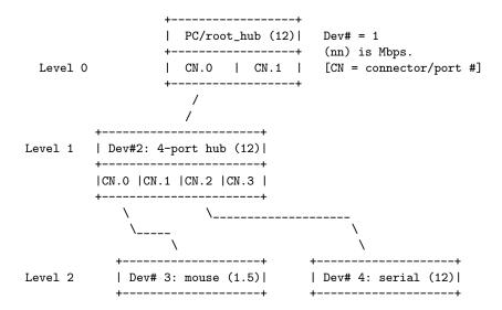
Or, in a more tree-like structure (ports [Connectors] without connections could be omitted):
