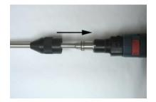
Screw the black sleeve onto the motor.
