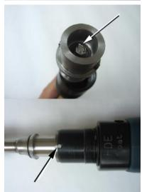
Re-attach shaft onto the motor.
