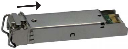
Figure 13: Installing an SFP transceiver
