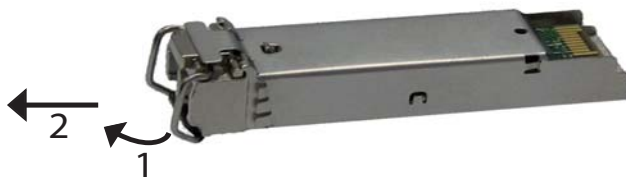
Figure 23: Deinstalling an SFP transceiver
