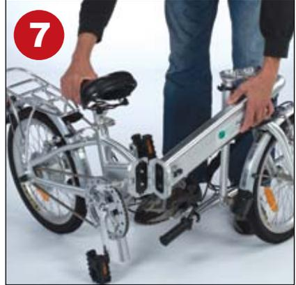
*Raise the kickstand and fold the the bike from the center hinge until collapsed tight.*
