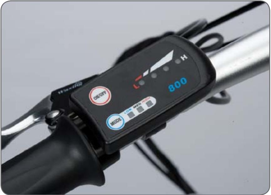
Figure 1. Power on, battery level indicator and PAS speed controller
