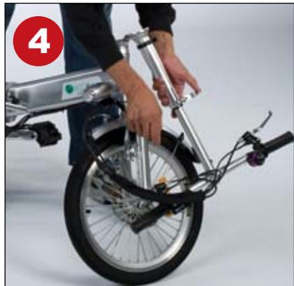
Lower the handlebars and adjust so that the brake grip and handle align to the center of the wheel hub, retighten the folding post clamp.
