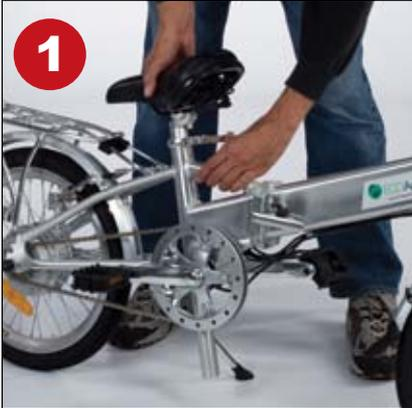
Standing beside the bike, loosen the seat post and lower the seat turning in to a reverse position facing backwards. Retighten the post clamp.
