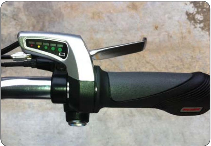
Figure 2. Slowly rotate the throttle towards you to engage the motor, rotate throttle away from you or engage brake to reduce speed.
