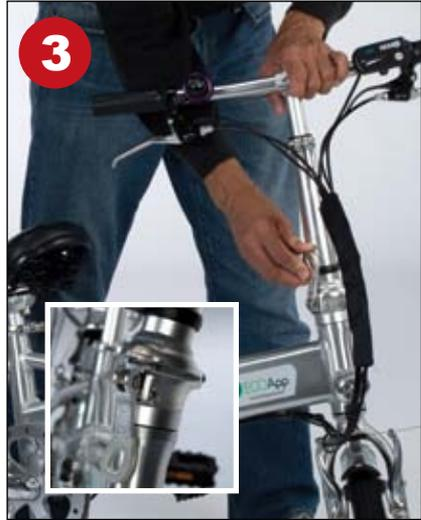
Next, loosen the folding post clamp located just above the front light on the front bike stem.
