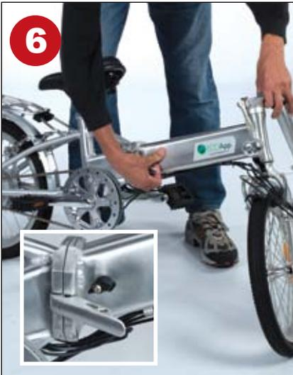
*Unclip the the the folding hinge, and leave open.*
