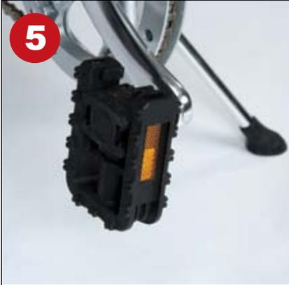
*Collapse the pedals by pushing in and turning them. Turn the pedal so that the pedal on the left side (chain side) of the bike is vertical to the ground.*
