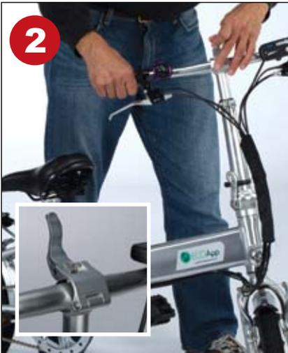
Loosen the center handlebar clamp and rotate so that the brake handle is facing the ground. Re-tighten clamp.
