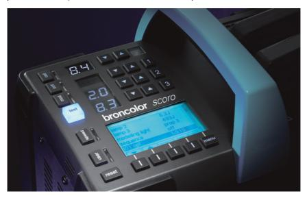
The brightness of the user interface can be automatically or manually\* dimmed dependent on the ambient light. See LCD setting function "Brightness display" (section 13.20).
