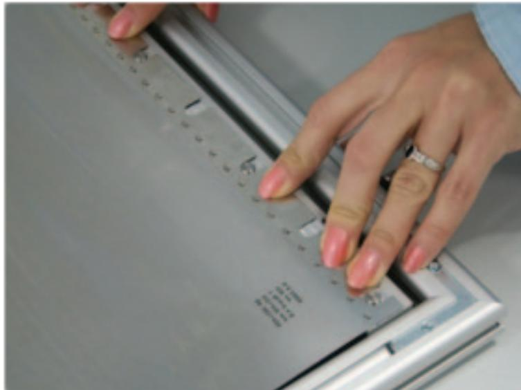
**9.** Close the front stretching bar with the front holding bar
