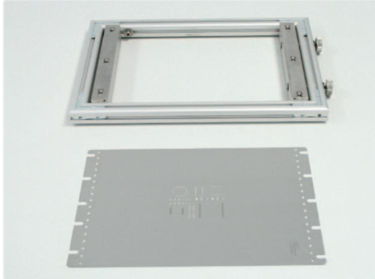
2. Using the two hexagon-headed screws, attach the rear bar according to the stencil length. Tighten them (the rear bar must be parallel to the rear frame profile).
