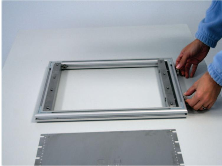
4. Remove the holding bars from the front stretching and rear clamping bars.
