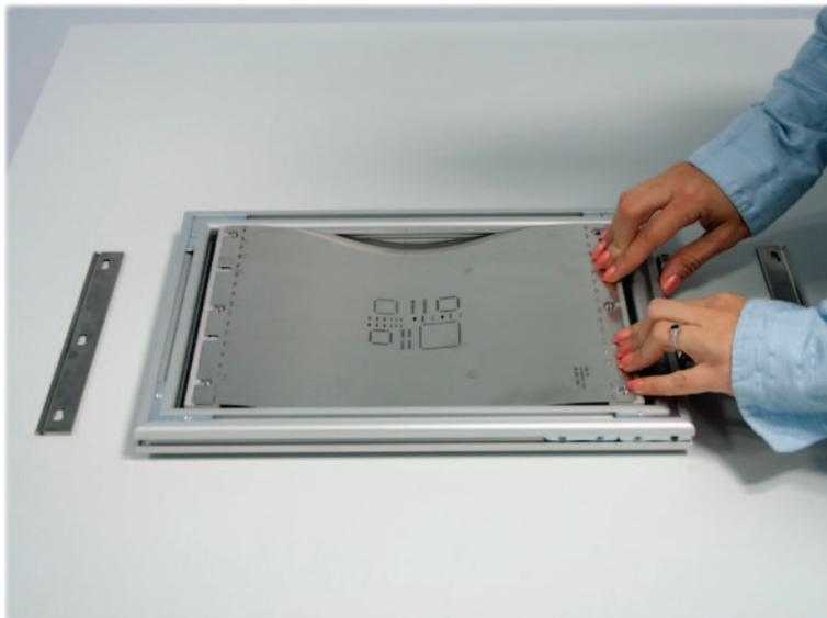
7. Close the rear clamping bar with the rear holding bar
