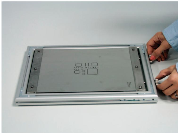
11. The gap between the locker on the stretching screw and the bar should be approx. 3 mm for the required working tension.
