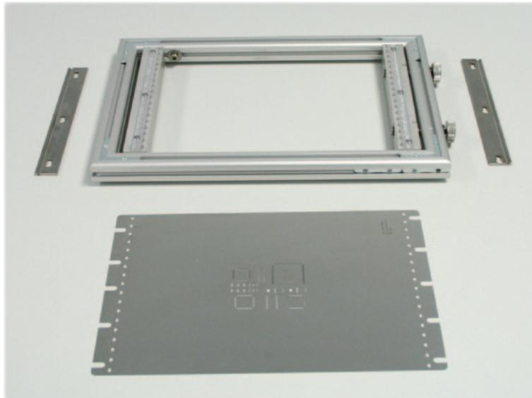
6. Place the stencil onto the pins on the rear clamping bar.
