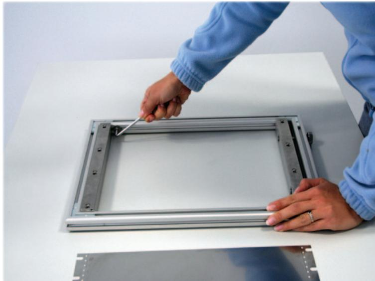
3. Unwind the stretching screws from the stretching units by about 10 mm.
