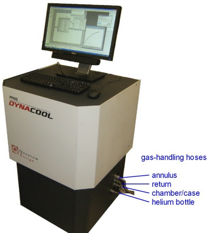
Figure 2-5. Front view of Pump Cabinet.
