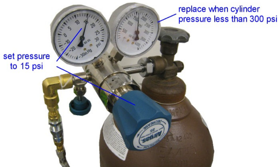
Figure 2-9 Helium gas bottle with regulator.
