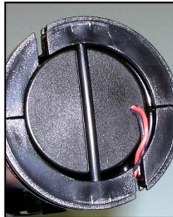
Downward force (see red arrow) may be required on battery end to get the pin started.
