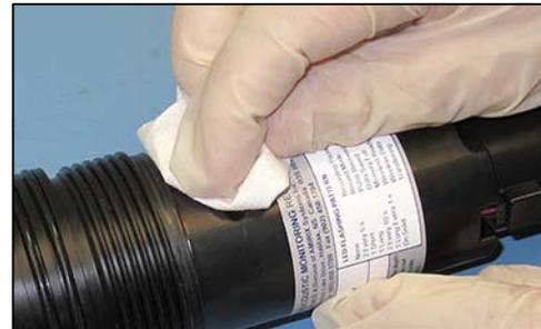
Place the receiver on a clean surface so the O-rings remain debris and damage free.
