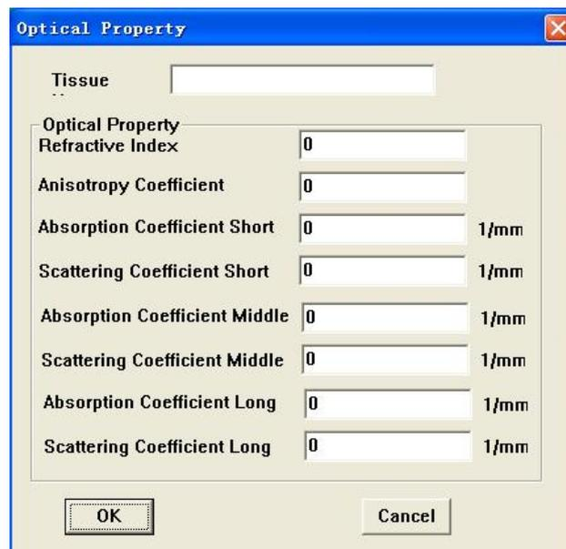
Figure 21-2. Set Optical Property Dialog for Multiple Spectrum in MOSE
