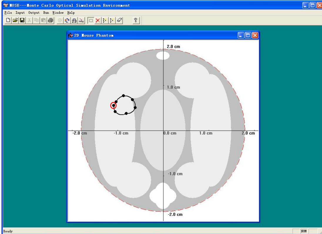
Figure 12-7-1. Delete an Anchor Point
