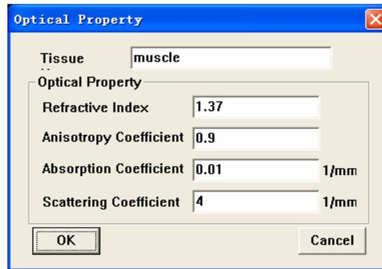
Figure 21-1. Set Optical Property Dialog for Single Spectrum in MOSE
