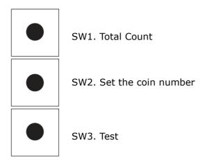
1. If you want to check the total amount of tests, press SW1 and the display window will show the test.
