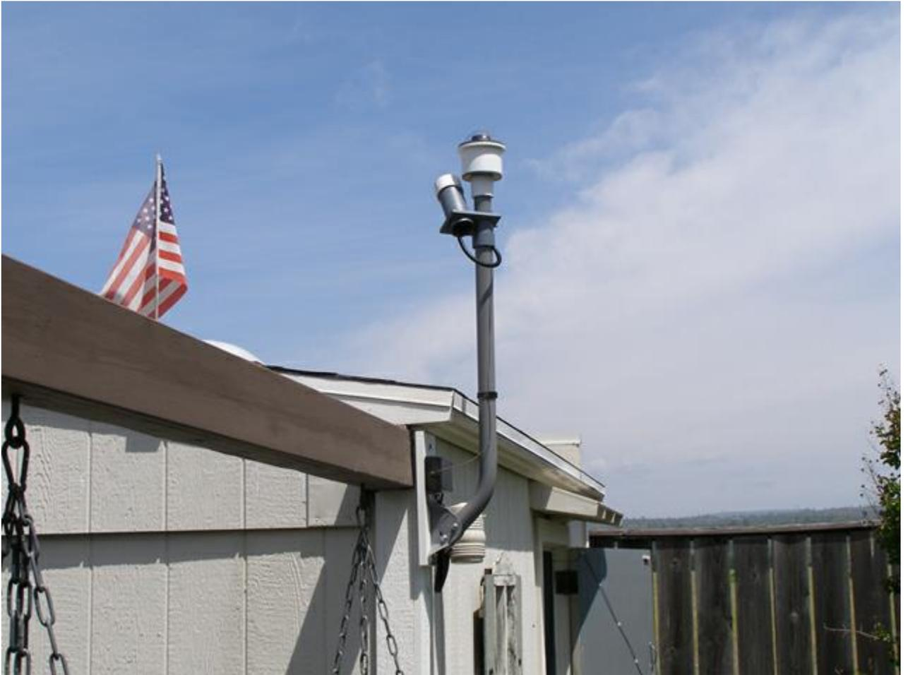
Choose a location for mounting the camera that is as high as possible to avoid obstructions near the horizons. An adjustable mask is incorporated into the camera to block unwanted light on the horizon as needed. The camera can be mounted on a standard 1.66" diameter satellite dish mount such as the [Winegard DS3000](#) or on a standard 1-1/4" diameter PVC pipe. Orient the marks on the camera housing so that they are pointing to North if desired.
