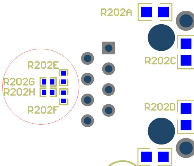
Settings of solder bridges are shown below. To establish state closed solder bridges (0 Ohm 0402 resistors) must be installed.
