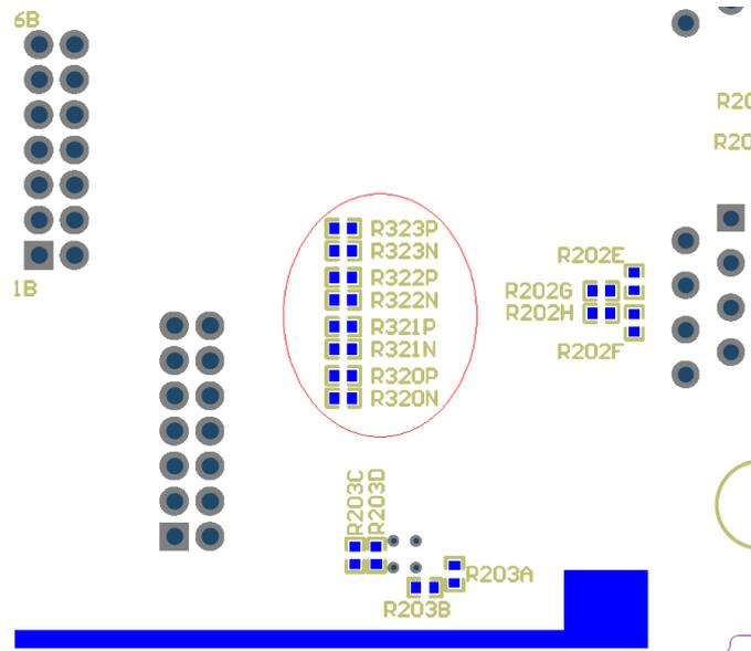
Routing table and settings of solder bridges are shown below. To establish connections to appropriate I/Os of Zone3 connector the corresponding solder bridges (00hm 0402 resistors) must be installed.
