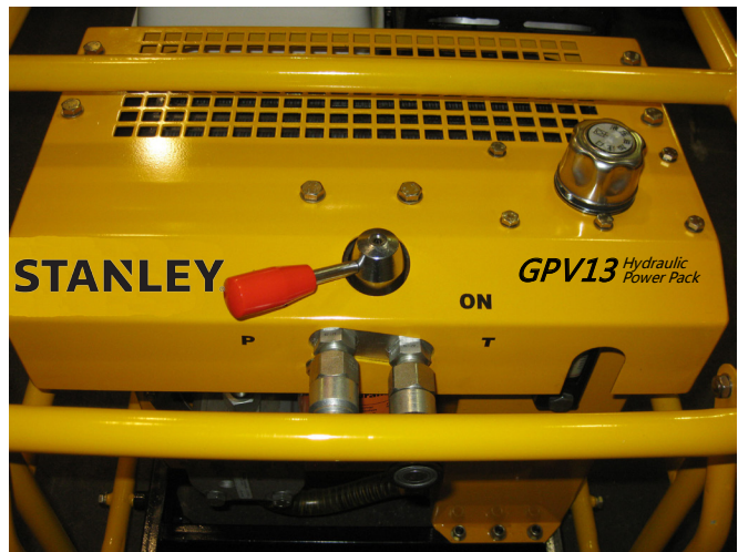
Figure 2. Panel Control Valve
