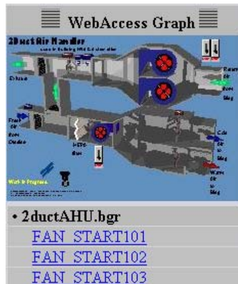
Figure 1.30 – typical THIN CLIENT Graphic Display with control tags (2ductAHU1.bgr).
