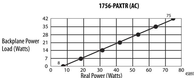
Apparent Power (Watts) = Transformer Load (VA) = Real Power (Watts)
