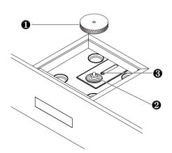
The TL3N's stabilizer is heavy, with a diameter of 7cm and weighing 330g. Hold the edge steadily when you place it on or remove it from the turntable. Dropping the stabilizer may damage it and decrease playback accuracy, so handle with care.
