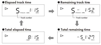
**NOTE:** Total remaining time and total elapsed time will not be displayed when program mode and/or repeat mode are active.
