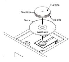
**NOTE:** Make sure you place the disc on the turntable with the label side facing up, and place the stabilizer on the disc before closing the CD door. The TL3N may be unable to read the disc unless you place the stabilizer correctly. Use only the provided CD stabilizer. Do not use commercially available stabilizers.
