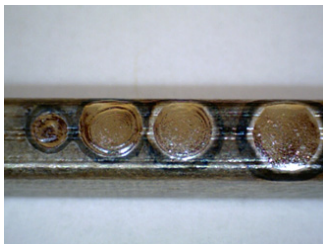
25 Joules with 0, 2, 4, 8ms weld length.
