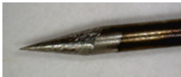
Electrode condition greatly affects power transfer and also weld properties (see above discussions). Left: A perfect electrode. Right: An electrode in poor condition with metal contamination.
