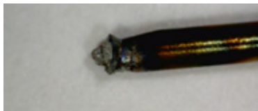
Electrode condition greatly affects power transfer and also weld properties (see above discussions). Left: A perfect electrode. Right: An electrode in poor condition with metal contamination.
