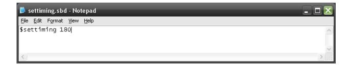
**180** = **IRD Check** interval is the number of minutes between Kilo's message checks, and GPS transmissions. The Kilo will wake up and check for messages (new instructions) at the Iridium Gateway based on this setting.
