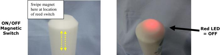
A flashing green LED indicates the device is in the process of powering up, continue to swipe the magnet until you see a solid green LED. A solid green LED indicates that the device is powered and operational.
