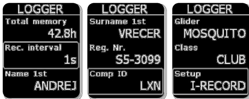
To change the text string, press the enter button and a cursor will appear. Using the up and down button change the letters. The left and right buttons move the cursor position in the text string. **The entered string will end behind the cursor when enter button is pressed.**
