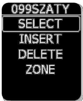
Pressing the Enter button while the white frame is around a TP name opens the TP edit menu. Use **select** to select a new turn point, and replace the existing point of the task. **Insert** will insert a new turn point one position higher. **Delete** will delete the existing point. **Zone** allows the creation of the sector geometry as specified by the task sheet. Every sector consists of two angles and two radii. Further inputs are zone orientation and Auto Next as discussed above.
