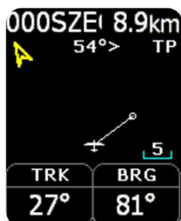
On this page the pilot will find basic information about navigation and also any TP stored in the internal TP database can be selected. In the top left corner the TP name is displayed, followed by the distance. The yellow arrow is a North indicator. In the central upper position steering information is shown. On the bottom of the display there are two navigation boxes that show track and bearing. Navigation is always track up.
