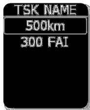
**LOAD TSK:** Transfers task from SD to device. Pressing enter button will show a list of **first 20 \*.cup** formatted files in the LX/TP directory on the card. Selecting file of interest will then give you list of **first 5** listed tasks in selected cup file. Select task which you wish to upload and transfer of task is completed.
