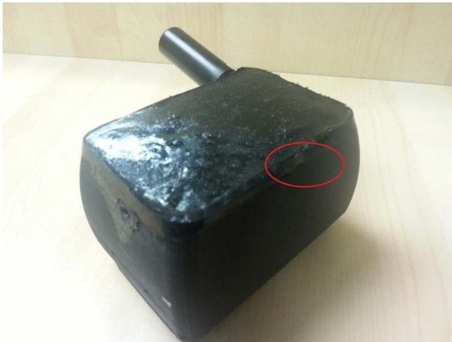
To know if the unit is off, simply place the magnet on the unit while the unit is still attempting GPS and sending the data via Iridium. If the magnet is placed on the correct spot, those emails with GPS data updates will stop coming and no more data will be placed onto the web. This means that you have placed the magnet successfully and the unit is off.
