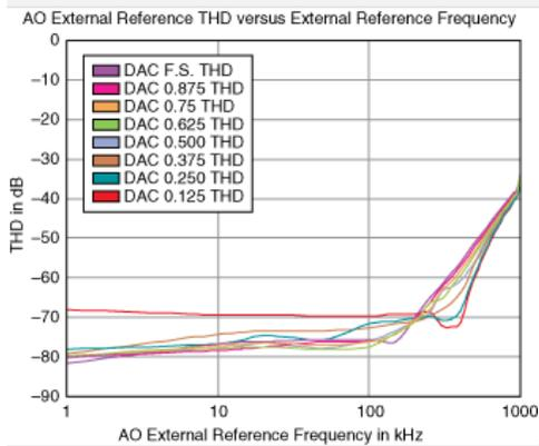
**NI DAQCard-6715 AO External Reference THD versus External Reference Frequency**
