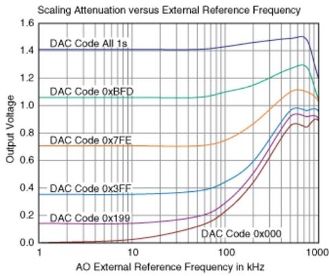
**Note** (NI 6711/6713 Only) External reference input is always a 1.414 V peak-to-peak sine wave.
