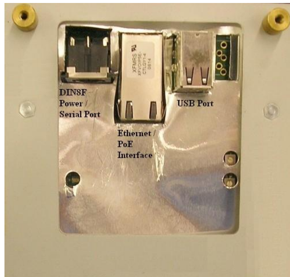
Figure 3—Connector Location—Rear of ScanVue®
