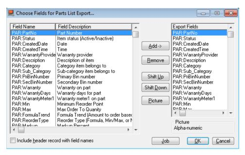
Choose the fields on the left that you want to include in the export file. Press and hold the CTRL key to select multiple fields or the SHIFT key to select a range of fields and press the "Add" button. To remove a field from export fields, select the field and press remove. You can shift the order of the fields by pressing the "Shift Up" and "Shift Down" buttons.
