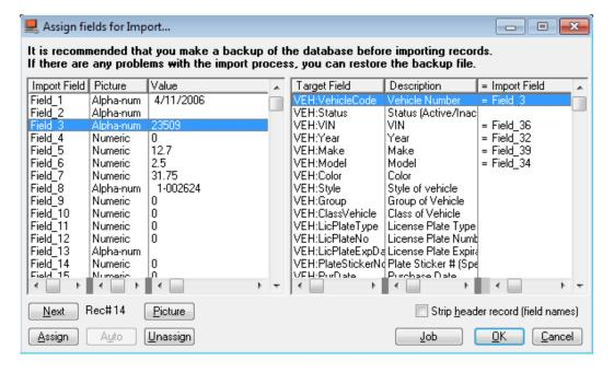
Choose the field from your import file on the left and then choose the target field on the right that you want to assign to. Press the "Assign" button to assign the field from the import file to the target database field. Press the "Unassign" button to un-assign the field.
