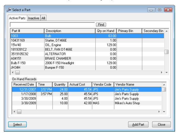
When you select a part manually, by default the selected quantity will be checked out sequentially in First in First out (FIFO) order. You can check out a specific inventory part by highlighting the part and the specific on hand inventory record. If the quantity chosen is greater than the selected on hand record, the system will remove the remaining quantity in FIFO order.
