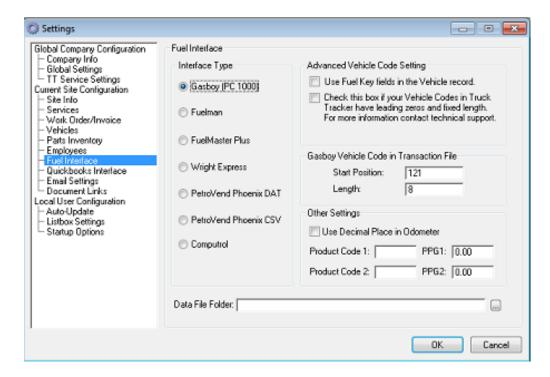
Select which system you're using, and then type the path of the **folder** (not the data file itself) where your fuel data is located. Alternatively, you can browse to this folder by clicking the ellipse button and navigating to the folder.
