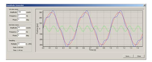
The amplitude is given in "counts" which is the metric of the positioning sensors. One count corresponds to one micrometer. Please note that the amplitude here denotes the displcement between the sensor and magnetic tape, the corresponding total travel of the voice coil will be different and has to be calculated.
