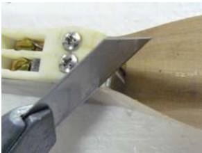
Cut the Teflon at the end of the end block till the table is reached.
