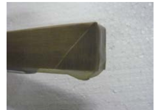
Make sure the Teflon is placed without wrinkles, they will influence a proper seal result.
