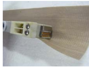
Then roll over the seal bar while pushing the seal bar to the table.
