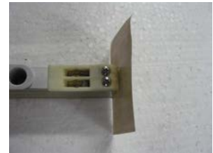
Fold the remaining Teflon up and push it against the end block.
