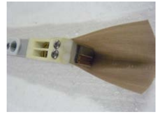
Then stick the Teflon to the other side. Prevent crinkles they will influence the seal result.
