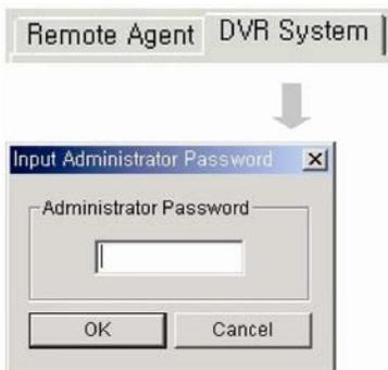
Click DVR System Setup Tab, password Input window opens After Entering Password, Setup Windows Pop-up.
