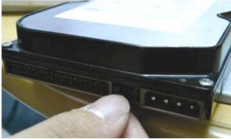
To setup HDD as Master or Slave refer to explanation (legend) on surface of Hard Disk.
