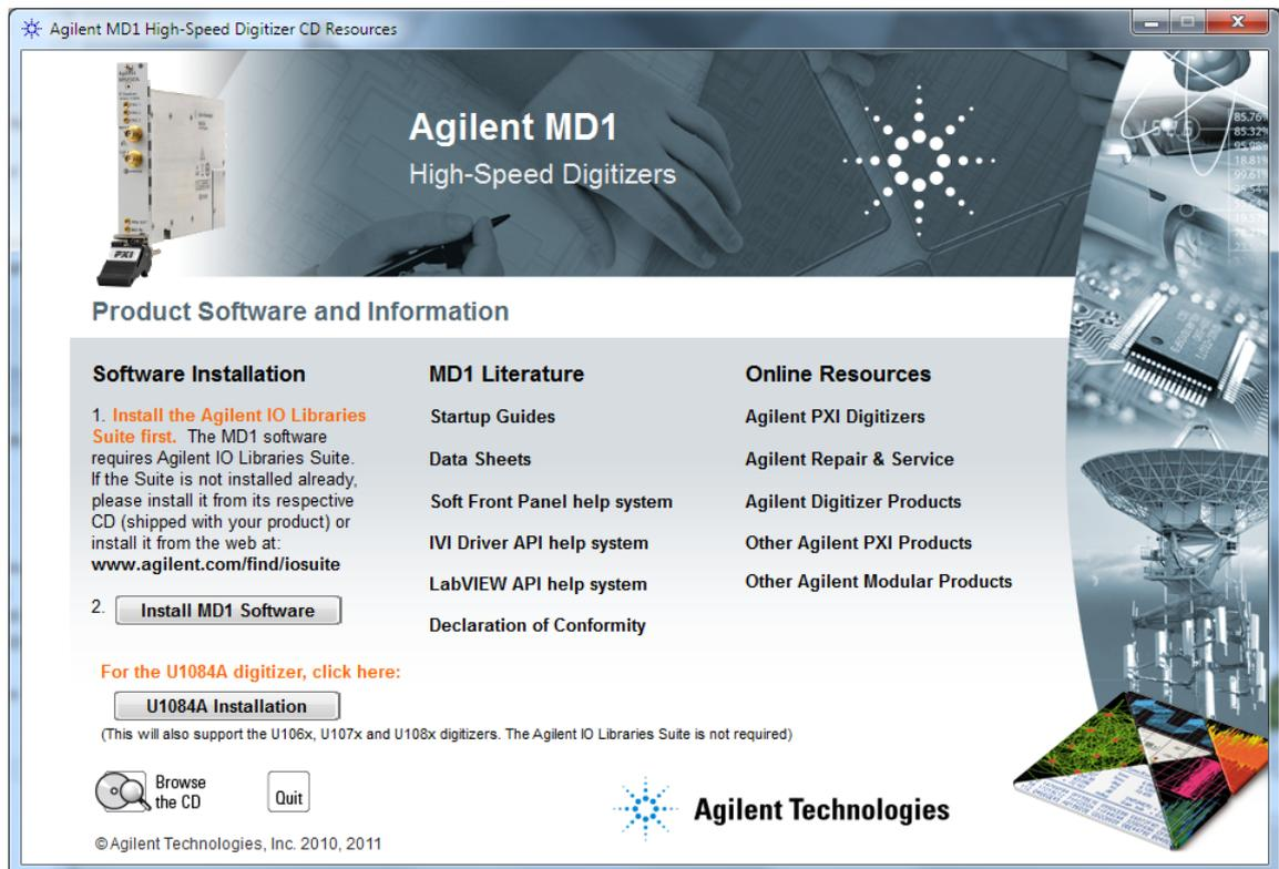
2. The 'U1084A Installation' button provides the option to install the U10xx Digitizer products package to your PC. This includes Device drivers, Soft Front Panel applications and documentation for the Agilent Acqiris 8-Bit digitizer products which are covered by this manual.
