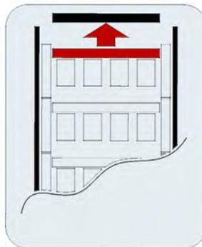
Insert the marker cards into the loader so that they are touching the end stop.
