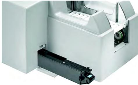
4. Place the full ink collector unit into the provided bag and dispose.
