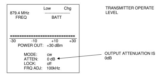
NOTE: The transmitter output power at the BNC is +30 dBm (1 watt) when the attenuator is set to 0 dB.
