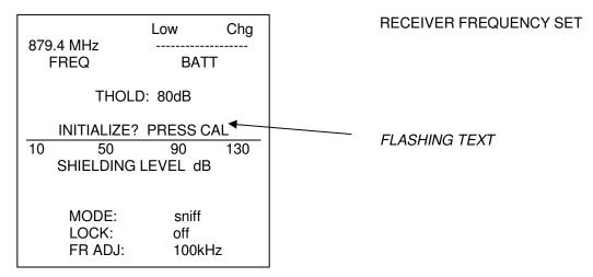
NOTE: The "INITIALIZE? PRESS CAL" warning will flash until a system level calibration is performed.
