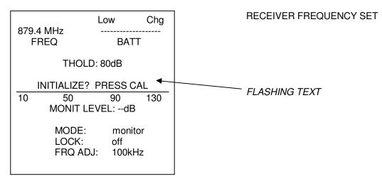
NOTE: The "INITIALIZE? PRESS CAL" warning will flash until a system level calibration is performed.
