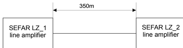
Fig. 2: Cabling without splitter
